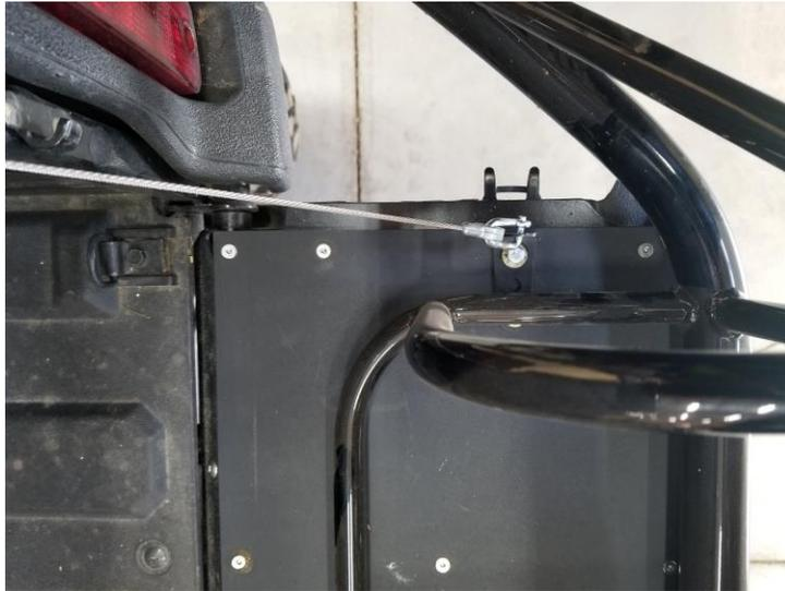
**(Please note the right side clearance from the extender to the tailgate bracket is larger in order for the extender to swing open toward the passenger side of the machine and clear the bracket)**
